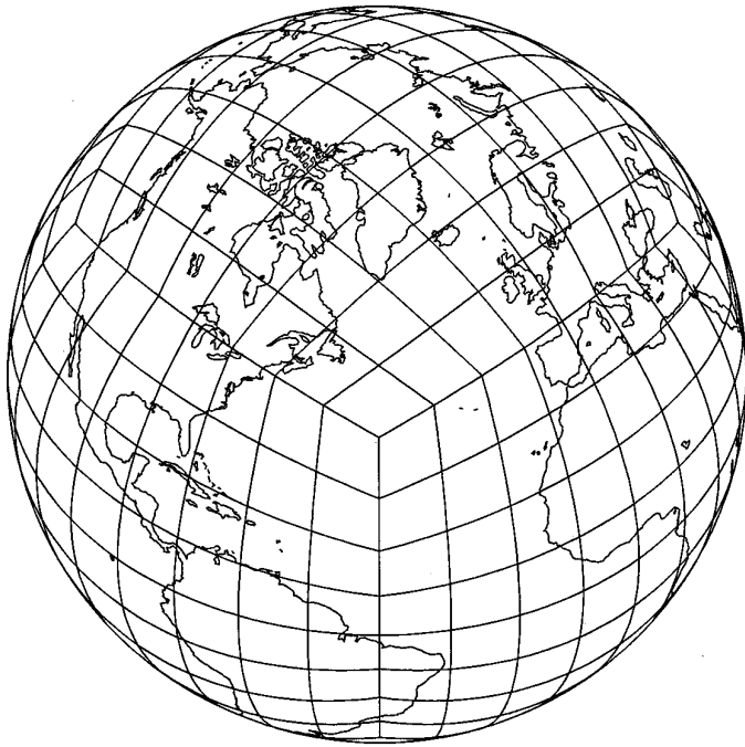
FIG. 1. The cube projected onto the sphere. Each of the six faces of the cube has been divided into an 8 \times 8 array of elements.
